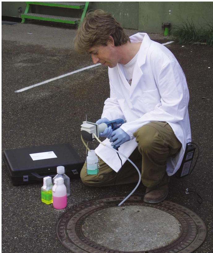
Vampire in use in the environmental protection sector for sampling from narrow openings and at substantial depths.
