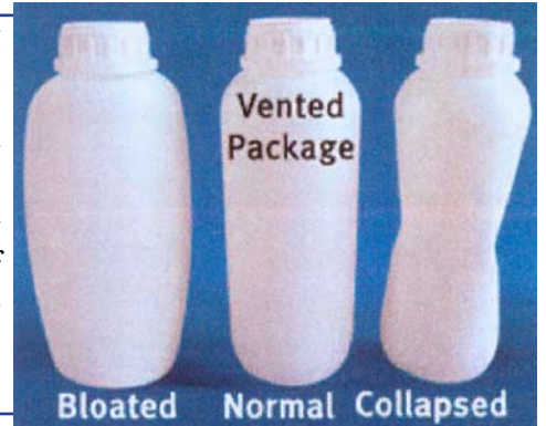
Bottles on the left & right are examples of packaging that should be using vented caps.
