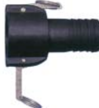
800560: Schutz camlock 2" female x 2" hose tail, with locking arms
